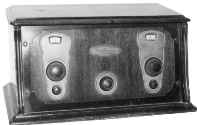
FREED-EISEMANN MODEL 30 – The Freed-Eisemann Corporation of New York manufactured this 6-tube battery set in 1926. It operates with the Neutrodyne circuit using two tuning dials. (Clark Trissell – Lincoln, NB)
